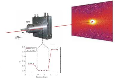
FIGURE 1: Illustration of the 1-2 plane shear cell in the neutron beam allowing for gap-resolved studies. The graph shows the recorded and predicted transmission as a function of beam position along the 2 axis using the 0.6 mm slit.
